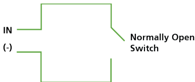
Figure 10: Normally Open Input Connection
