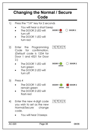
• The system will return to Normal mode (Default Secure code is 3838 for Door 1 and 8383 for Door 2.)
