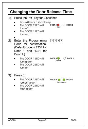
**NOTE:** This is a 4-digit code. The first digit signifies whether the unit is being used for fail secure (factory default setting) or fail safe operation. The second digit signifies the length of time in minutes the tamper alarm will sound. The last 2 digits signify the time the door release will be activated (from 01 to 99 seconds).
