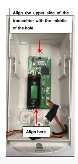
Step 3. Connect the wires and fix the wires as the pictures shown below.
