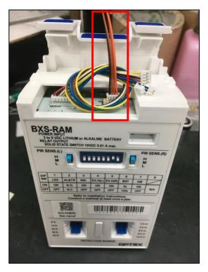
Step 4. Turn the BXS-RAM around. Use the wires to make a loose knot and thread the wires' end into the circles. Apply a foam tape to fill in the gap as the picture marked below. Align the transmitter in the middle of the back cover as the picture shown below.
