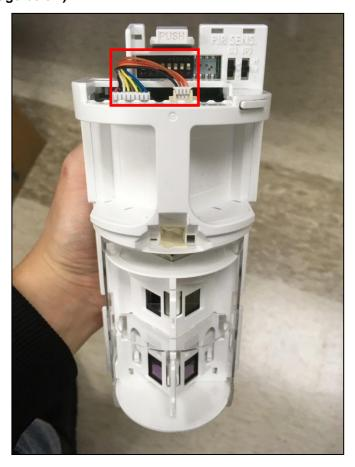
Step 3. Fix the two set of wires onto WXI-RAM.
