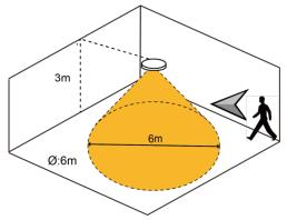
• When mounted on the ceiling, the PIR has better detection performance against horizontal movement.
