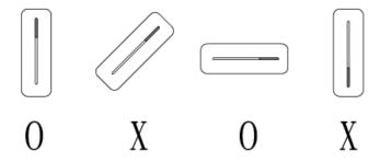
• The Garage Tilt Sensor should be mounted on the top panel of the garage door.
