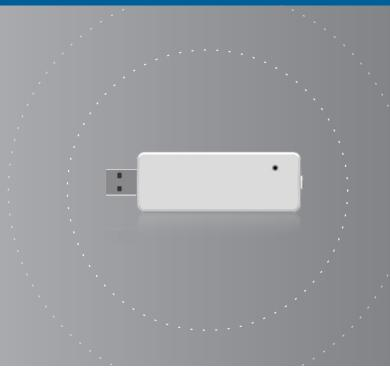
Climax Technology LoRa Dongle enables models from Hybrid Panel, HSGW and ESGW Series to employ the LoRa protocol as their reporting path, which can be an alternative when the main communication path fails. Through the LoRa dongle, compatible devices can enjoy long-range, low-power communications.
