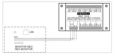
To activate the devices to be controlled, use the relay outputs 1 to 8, corresponding to the activations R1 to R8 of the monitor control screen. Relay outputs 0 and 9 are not used.
