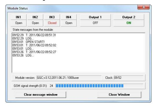
The monitoring window can be opened by clicking on the "magnifier" icon in the upper right corner of the main window. The icon is available only when the module is connected. This window indicates the current state of the inputs and outputs of the module, the module version, the module's internal clock setting and the GSM signal level.
