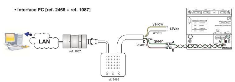
Note: The panels' address must be configured previously on the panels themselves (DISPLAY EXTRA)
