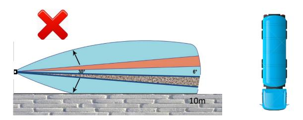
NB: The sensor can detect objects such as cars and /or trucks beyond the detection zone, Then avoid installing the sensor facing a vehicle passage or use the kunction bracket and tilt down the sensor to reduce the coverage area.
