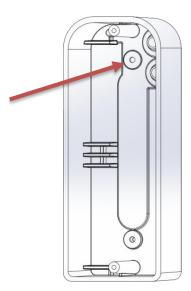
**5.** Replace the metric screw with those in the bag and insert the seals into the compartments as indicated
