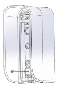
**13.** After the wiring and operation test close NAT sure that the seals and the O-rings are present and not damaged to ensure the integrity of the product.
