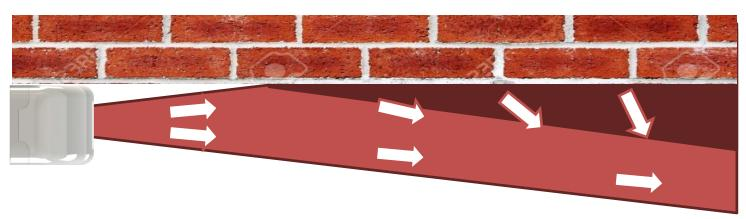
If the NAT sensor is applied along a wall, it is possible that the PIR detects an area of none interest that can generate more or less important reflections and false detections depending on the type of material present. In order to obtain a more precise and safe area of detection it is possible to apply the PIR LIMITER supplied which limits the angle of view of the sensor.
