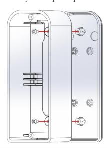
7. Check that the gaskets on the cap are correctly insert
