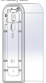
**4.** Drill the passage of the screw shown in the drawing
