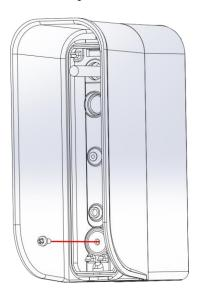
**10.** After the wiring and operation test close NAT sure that the seals and the O-rings are present and not damaged to ensure the integrity of the product.
