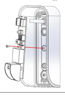
**9.** Drill hole in the rubber nut and slide inside the cable and insert then in the Nat base
