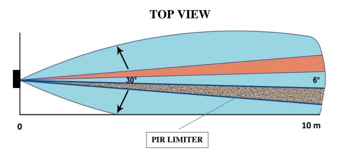
**NB:** Avoid positioning the sensor near mobile objects such as cloths or plants within the detection area
