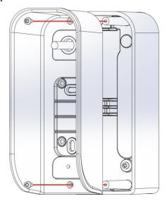
**10.** Insert the Nat base hook into the cap compartment as shown in the figure
