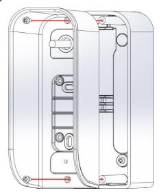
7. Insert the Nat base hook into the cap compartment as shown in the figure
