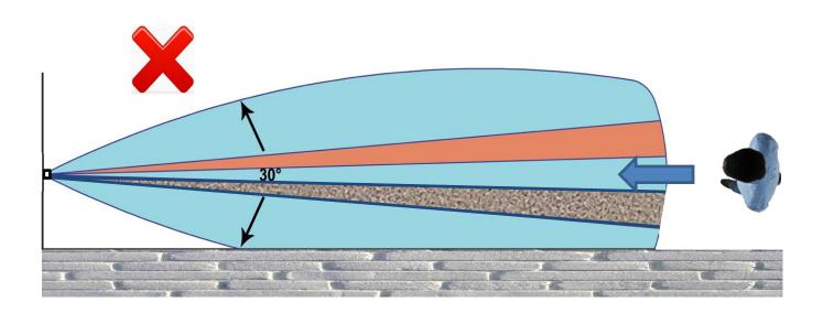
The sensor is designed for cross-tracing detection. Properly use the PIR Limiter for proper detection (Chapter 8).
