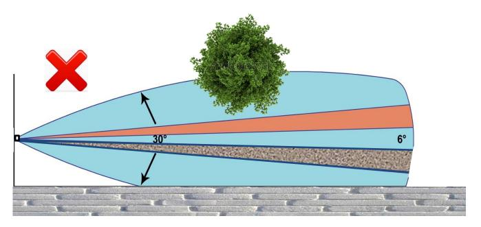
NB: Avoid the presence of plants, air conditioners and moving objects in the detection area
