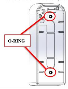
**6.** Screw the battery case at plastic plate
