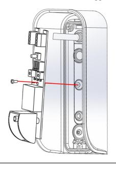
**6.** Drill hole in the rubber nut and slide inside the cable and insert then in the Nat base
