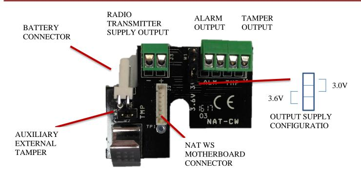
It is possible to power the 3.6V or 3V radio transmitter by using the same power as the NAT WS Sensor.
