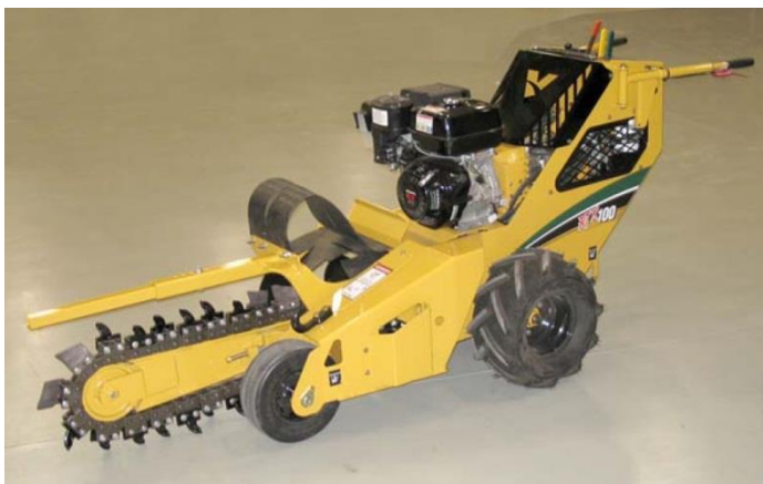
Picture 5: The ground trencher and the possibilities
