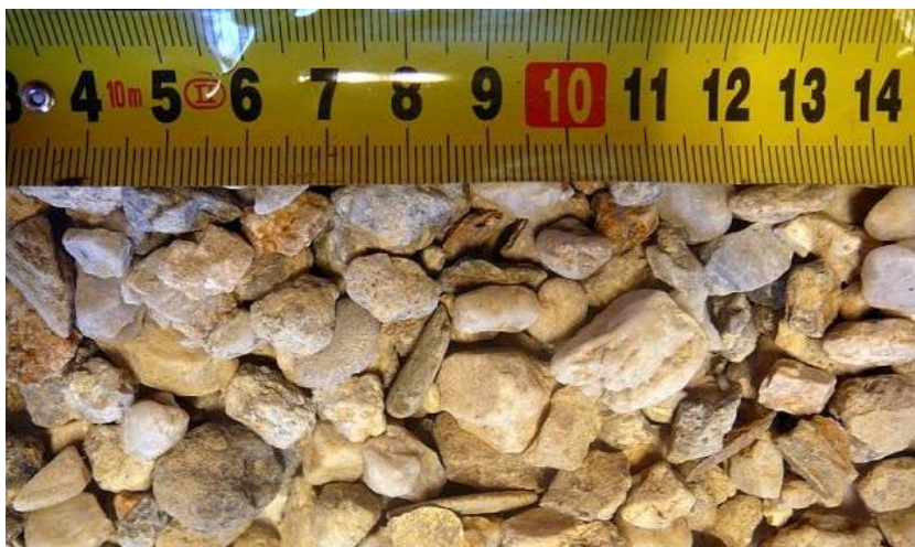
Picture 6: Gravel sorted when wet, fraction 8/16
