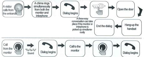
Dialog between the interphone and camera is possible only when the visitor's image is visible on the monitor screen.
