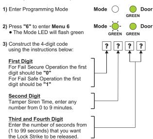
For example 0 5 1 2 means Fail Secure Operation, with a 5 minute Tamper Siren Time, and a 12 second Lock Strike release time.
