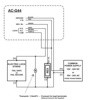
Wiring the Auxiliary Input and Output
