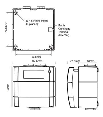
Ensure the cable entry holes are in the vertical plane, with either the single or double entry holes at the top.
