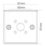
The FC420CP-I may be fitted to a standard (surface mounting) call point back box which is available separately.
