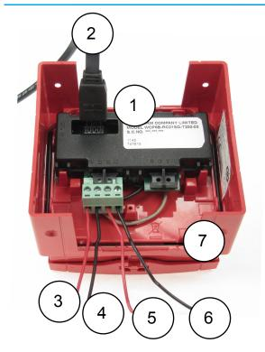
The FC421CP-I has a factory set (invalid) address of 255. The FC421CP-I is field programmed with the address prior to installation using a FireClass address programming tool. The associated ancillary programming lead plugs into the programming port.
