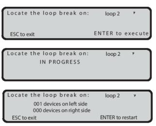
**Note:** During the locate loop break procedure all the detectors power down. At the end of the procedure, a full loop initialization is executed. The devices not in the configuration are not found.
