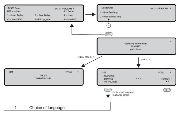
Figure 6: LCD screens sequence for downloading language strings from USB key at first panel power-up
