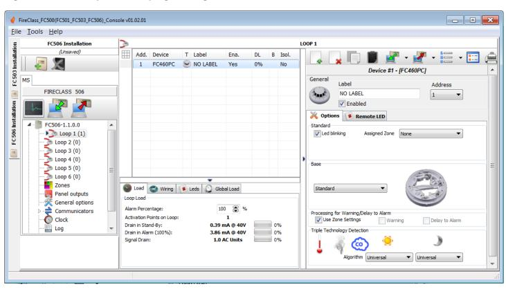
Figure 11: Detectors parameters programming window
