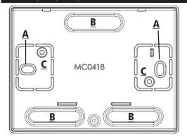
Knock out (where necessary) the points B, for cable entry. Fix the bottom of the box plastic, with 2 screws at points A Fix the board at points C
