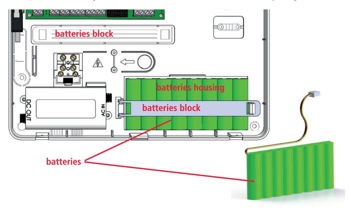
Fix the battery in housing with plastic blade (battery block) in fig.
