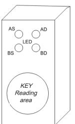
IMPORTANT: individual LEDS for each type of reader can be freely associate with each partial. Therefore, you can have readers with LEDs that activate different programs depending on their position in the site to be protected
