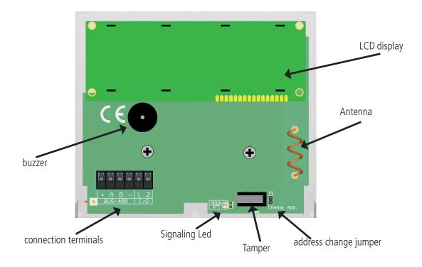
**K-Radio 800** must be connected in to the + - A B terminals in panel, for enabling the board go in peripheral menu from panel. **Reset hardware procedure:** it's possible reset the board directly from panel menu, but is possible reset direct on board:
