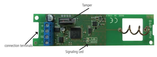
**EXPR800** must be connected in to the + - A B terminals in panel, for enabling the board go in peripheral menu from panel. **Reset hardware procedure:** it's possible reset the board directely from panel menu, but is possible reset direct on board:
