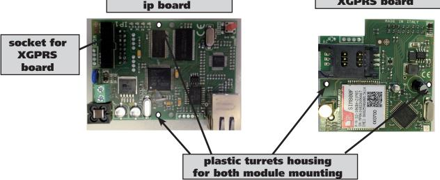
For fixing the IP1 module on the box of panel use the screw conatined in the panel screw kit, for connect use flat cable For fix X3/gprs module the same of IP1, in case of use both modules: fix for first IP1 module, after fix in socket the X3/gprs module with plastic turrets.
