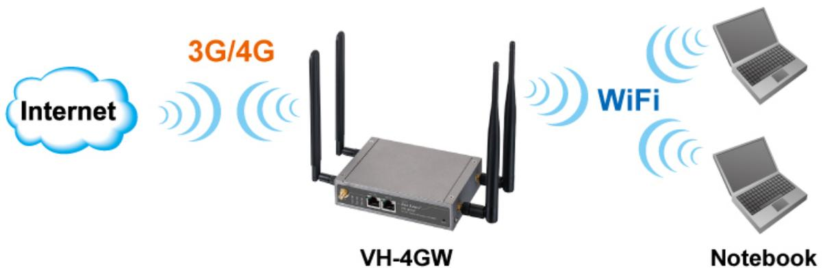
In this mode, this gateway is working as a WiFi AP, but also a WiFi hot spot. It means local WiFi clients can associate to it, and go to Internet. With its NAT mechanism, all of wireless clients don't need to get public IP addresses from ISP.
