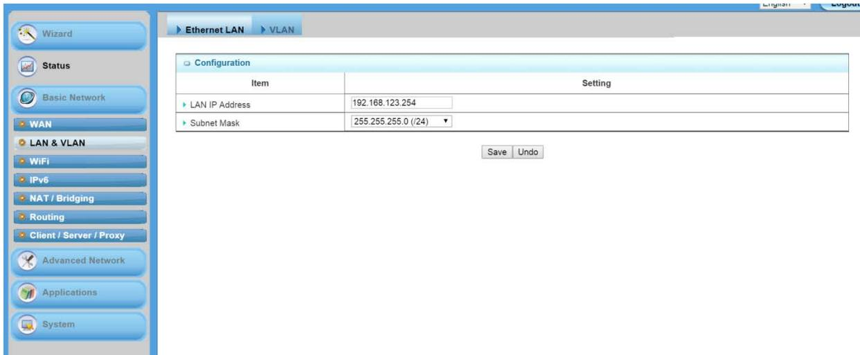
1. **LAN IP Address:** The local IP address of this device. The computers on your network must use the LAN IP address of this device as their Default Gateway. You can change it if necessary. It's also the IP address of web UI. If you change it, you need to type new IP address in the browser to see web UI. By default, LAN IP Address is 192.168.123.254.
