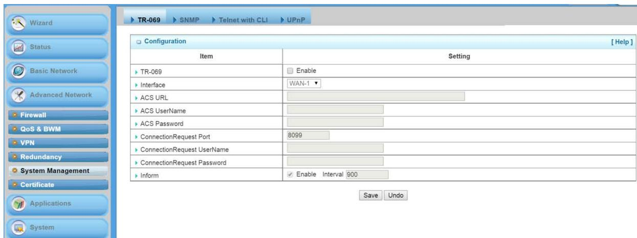
TR-069 is a customized feature for ISP; it is not recommend that you change the configuration for this. If you have any problem in using this feature for device management, please contact you're your ISP or the ACS provider for help. At the right upper corner of TR-069 Setting screen, one "[Help]" command let you see the same message about that.
