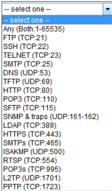
7. **Protocol:** Specify which packet protocol is to be filtered. It can be TCP, UDP, or Both.
