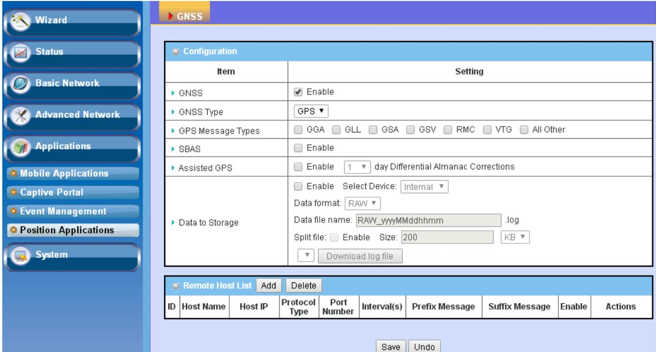
The screenshot shows the GNSS configuration interface. On the left is a sidebar with navigation buttons: Wizard, Status, Basic Network, Advanced Network, Applications, Mobile Applications, Captive Portal, Event Management, Position Applications, and System. The main area is titled 'GNSS' and contains a 'Configuration' section with the following settings:
