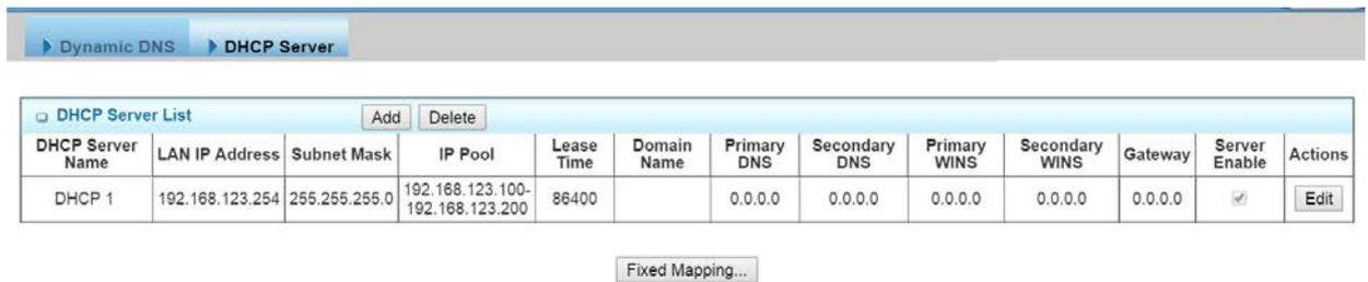
The screenshot shows a web interface for DHCP Server configuration. At the top, there are tabs for 'Dynamic DNS' and 'DHCP Server'. Below the tabs is a 'DHCP Server List' section with 'Add' and 'Delete' buttons. A table lists the DHCP server configuration:
