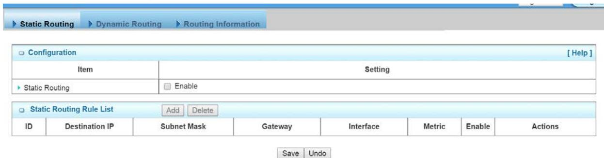
For static routing, you can specify up to 32 routing rules. The routing rules allow you to determine which physical interface addresses are utilized for outgoing IP datagrams. You can enter the **destination IP address**, **Subnet Mask**, **Gateway**, and **Metric** for each routing rule, and then enable or disable the rule by checking or un-checking the Enable checkbox.
