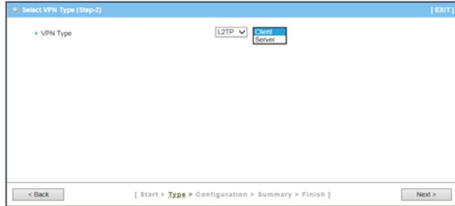
If choosing L2TP Client, please input tunnel name, IP/FQDN of L2TP server, user name & password, choose authentication protocol and MPPE encryption option. Please make sure these settings are accepted by remote L2TP server. Otherwise, L2TP server will reject the connection.
