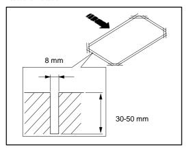
For installation of the loop cable use the number of turns indicated in the table.
