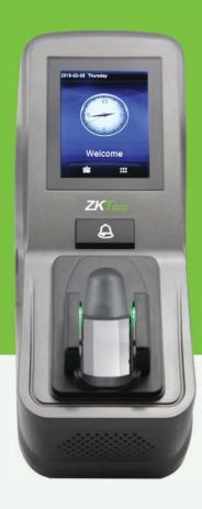
ZKTeco's first Finger Vein identification Access Control terminal. Ergonomic, intuitive and highly secured, V350 leads us to a new era for biometric application to security.
