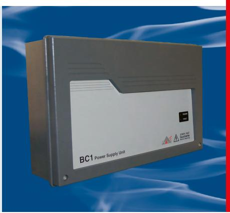
The Protec 9000/BC1 is a 24V dc 1A intelligent power supply and battery charger designed to be used in conjunction with two 12V 3.3Ah Sealed Lead Acid batteries. The charger continuously monitors various critical levels and gives a fault warning if any of the levels are out of specified limits.
