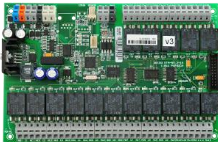
Quido RS I/O module with 16 outputs
