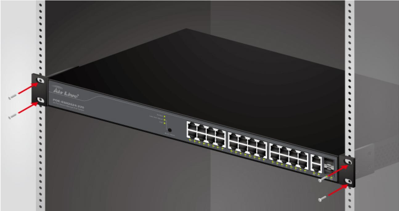
**Note:** For proper ventilation, allow about at least 4 inches (10 cm) of clearance on the front and 3.4 inches (8 cm) on the back of the Switch. This is especially important for enclosed rack installation.
