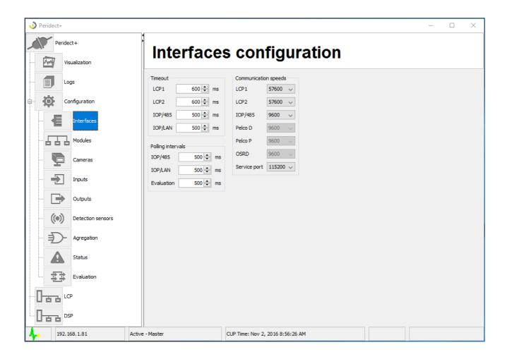
The two serial RS232 lines are used to connect the LCP line modules. The RS-485 is used to communicate via the MODBUS protocol, as well as usage of PELCO and OSRD protocols.
