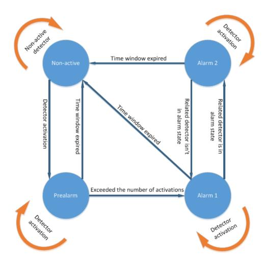
This picture shows the logic of event evaluation (the status automat) and the relation between the segment comparison mode can also be recognized.
