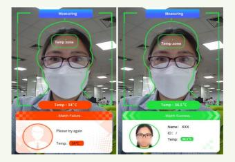
When the captured face is not added to the face database or the similarity is lower than the pre-defined value, it will display "Match Failure" and the box will turn red.
