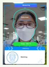
The system will measure the temperature and compare the captured face at the same time as shown below.
