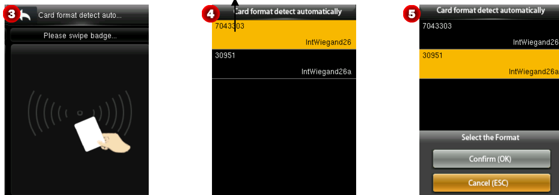
Card number obtained based on the IntWiegand26 format parsing
