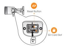
Note: Press and hold the reset button for 10 s to reset the camera.
