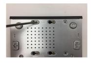
4. Turn the Device upside down and then fasten the screws.
