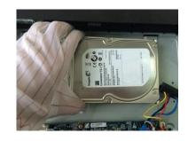
Place the HDD onto the Device.
