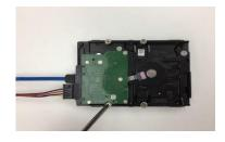
2. Connect the HDD cable and power cable to HDD, and fasten the screws in HDD.
