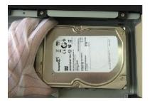
3. Put the HDD into the Device.
