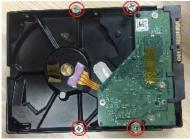
Fix the screws onto the 2. HDD, but do not be fastened.
