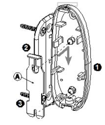
1. Place the base slots over the two bracket pins.
