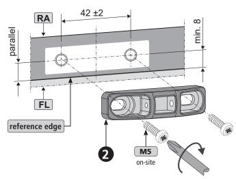
■ Screw the frame bracket ③ of BDB104 onto the casement (M5).
