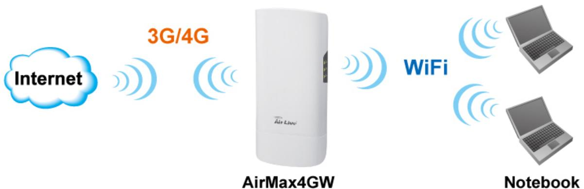
In this mode, this gateway is working as a WiFi AP, but also a WiFi hotspot. It means local WiFi clients can associate to it, and go to Internet. With its NAT mechanism, all of wireless clients don't need to get public IP addresses from ISP.
