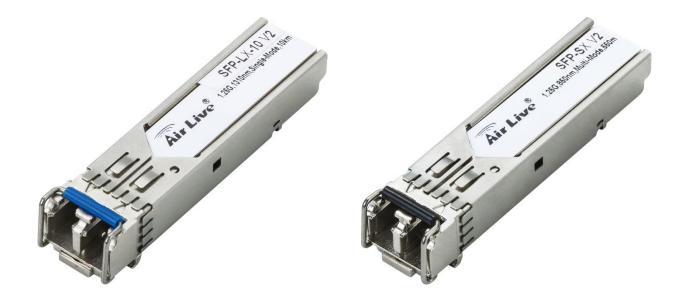
The SFP-LX-10 v2 is a high performance and cost-effective module for serial optical data communication applications specified for singlemode of 1.25 Gb/s. The module is intended for single mode fiber, operates at a nominal wavelength of 1310nm. The module is a duplex LC connector transceiver designed for use in Gigabit Ethernet applications and to provide IEEE802.3z compliant link from 125Mbps to 2.125Gbps applications.
