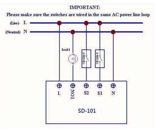
Fig 1. Assembling & Wiring
