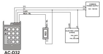
Figure 9: AC-D32 – Wiring the BL-D40 External Sounder
