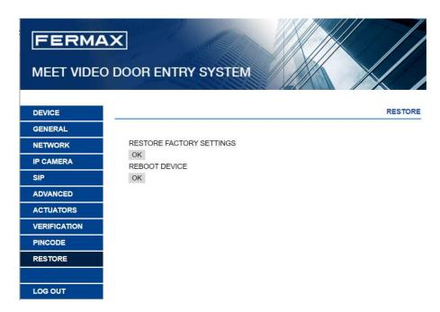
■ **RESTORE FACTORY SETTINGS:** The monitor will automatically turn off and start up with the factory settings:
