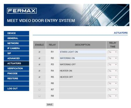
Indicate (ACTIVATE) the relays to be enabled and write the name or description that should appear on the monitor when you want to control any of them
