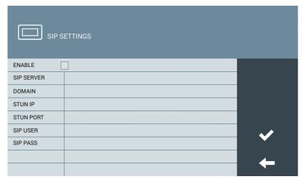
Use the on-screen keyboard to enter the SIP configuration data:
