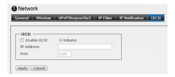
Enable the iSCSI and key-in server IP address and Port number. The disk of the server will be the storage in IP camera setting.
