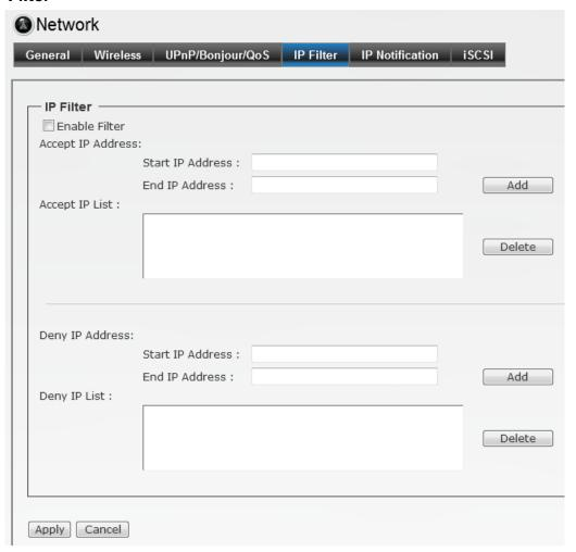
The IP Filter allows the administrator of the camera to restrict the users within a certain range of IP addresses to access into the camera. Select the **Enable Filter** option and assign the range of IP addresses that are allowed to access into the camera in the **Accept IP Address** field; or assign the range of IP addresses that are blocked to access into the camera in the **Deny IP Address** field.
