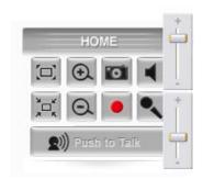
**Volume:** Click Speaker/ Microphone button to activate this function. Scroll the control bars to adjust the audio attribute.
