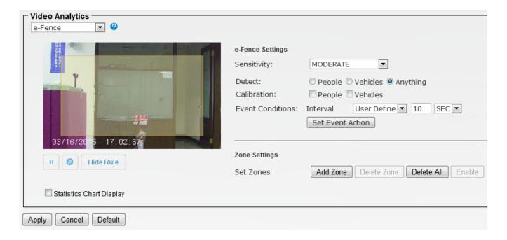
Select Sensitivity to set the detection sensitivity level. Higher sensitivity will make it easier to detect and less objects missing, but more misjudgments.
